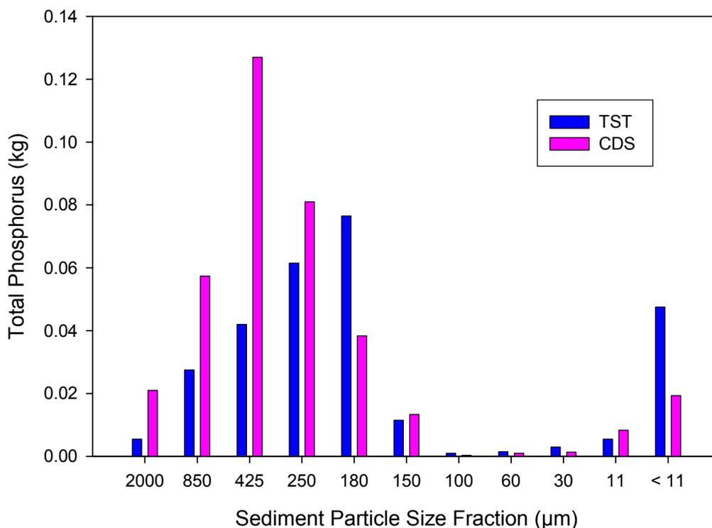
Figure 5-27. Size Distribution of Phosphorus Particles Removed from the CDS and TST Units.
