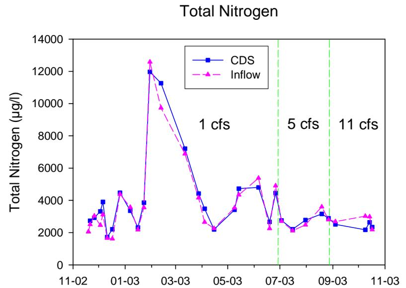
Figure 5-17. Concentrations of Nitrogen Species in Inflow and Outflow of the CDS Unit.
