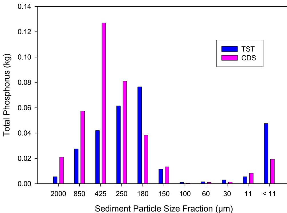
Figure 5-26. Particle Size Distribution of Suspended Solids Removed from the CDS and TST Units.
