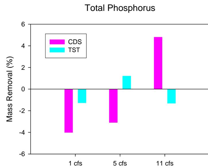
Figure 5-22. Comparative Mass Removal Efficiencies for Phosphorus Species in the CDS and TST Units.
