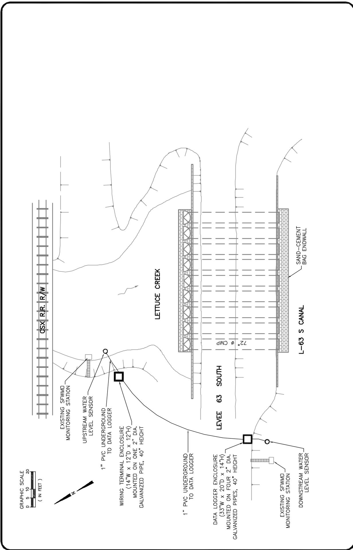
Figure 3-1. Locations of Initial Hydrologic Monitoring Equipment Installed at the Lettuce Creek Site.
