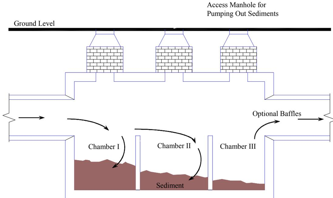
Figure 2-3. Schematic Diagram of Sediment Trap.
