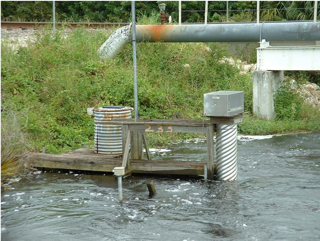
Figure 3-3. District Water Level Monitoring Station.
