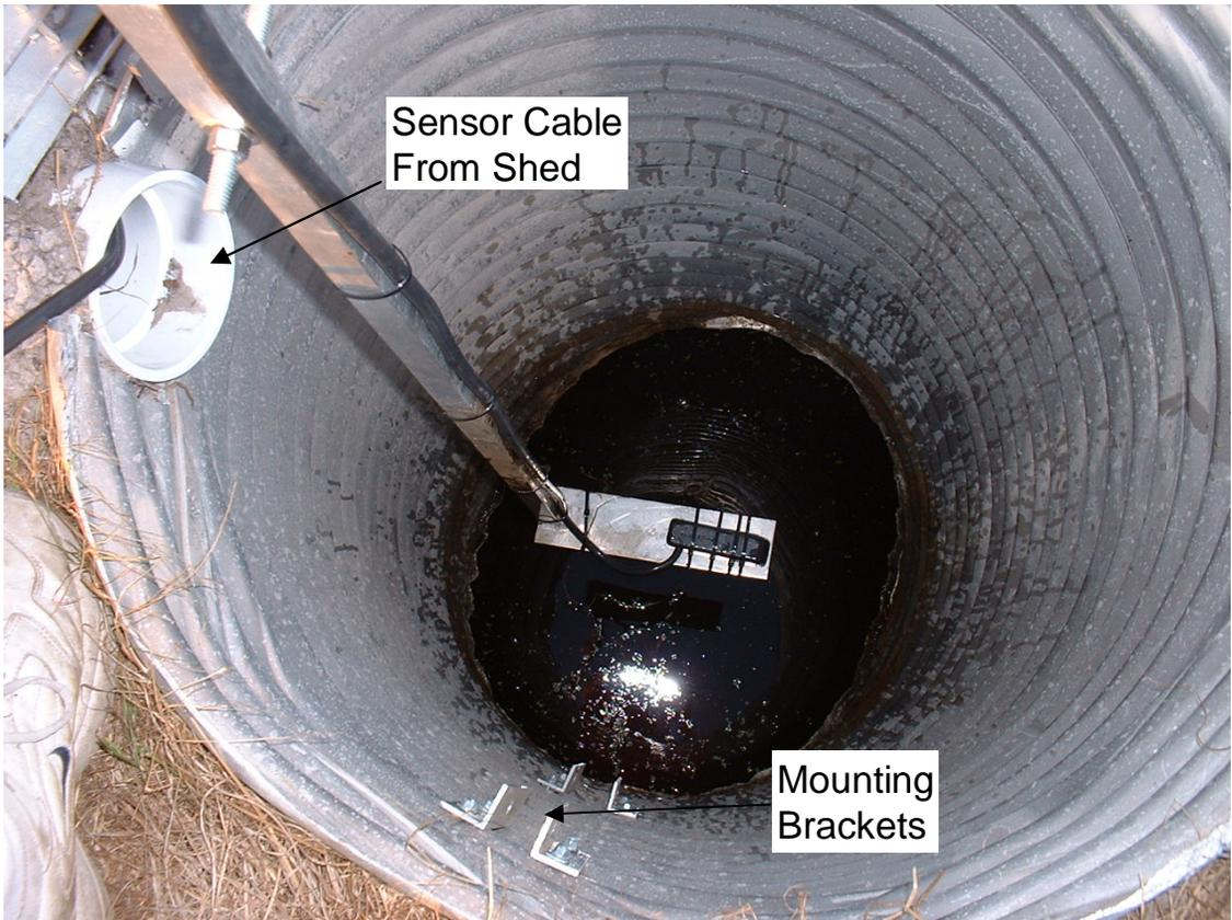
h. Riser Structure Used for Installation of Flow Probes
