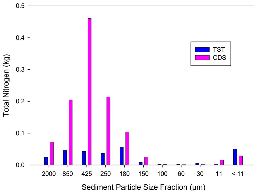
Figure 5-28. Size Distribution of Nitrogen Particles Removed from the CDS and TST Units.
