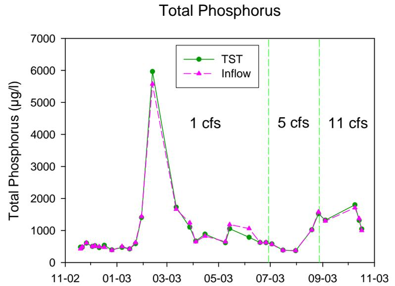
Figure 5-19. Concentrations of Phosphorus Species in Inflow and Outflow of the TST Unit.
