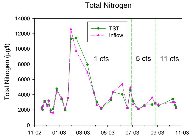
Figure 5-20. Concentrations of Nitrogen Species in Inflow and Outflow of the CDS Unit.
