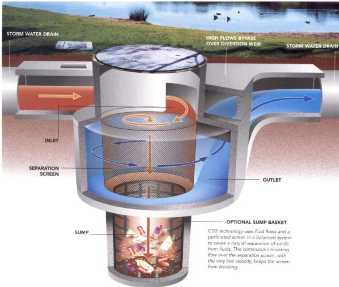
Figure 2-1. Schematic Diagram of CDS Unit.
