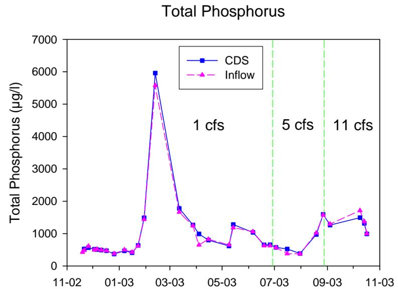
Figure 5-16. Concentrations of Phosphorus Species in Inflow and Outflow of the CDS Unit.
